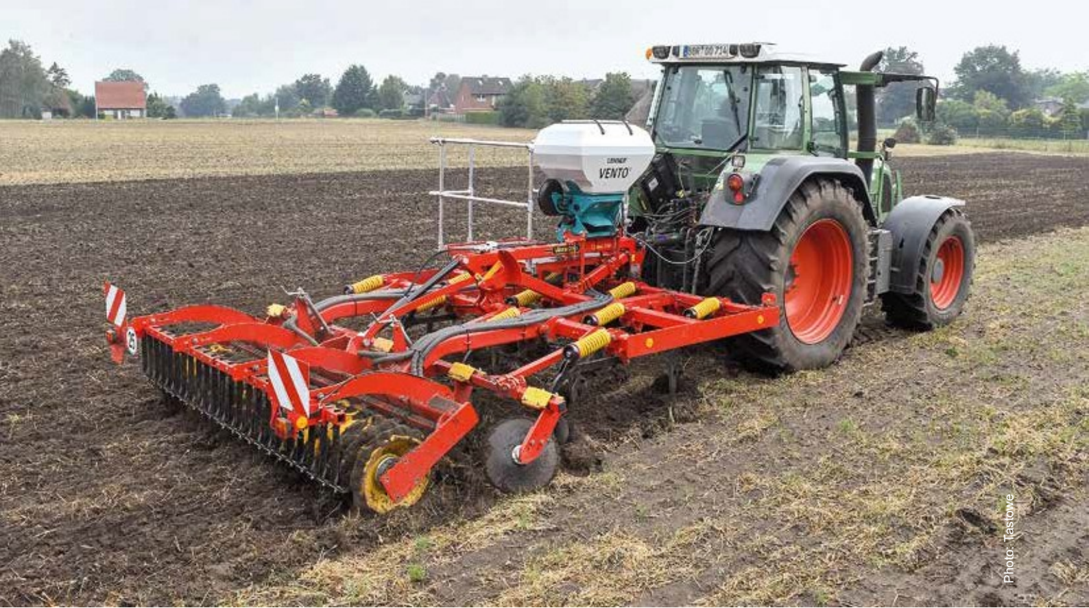
△ We used the Lehner Vento to sow catch crops after cereal, among other things. In the test, lateral distribution was good.
