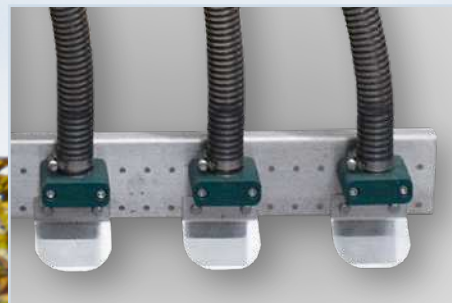
Hoses vertical and uniformly spaced for surface dispensing of seeds
