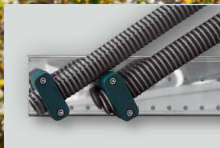
Sideways hose positioning for fertilising in rows
