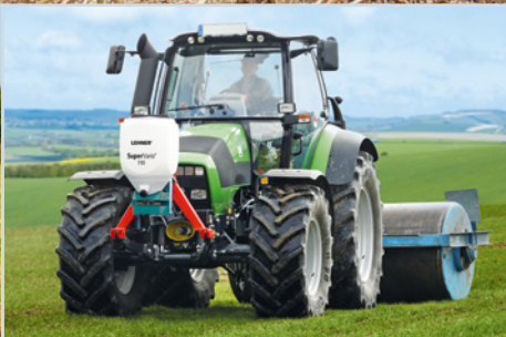
Reseeding grass in combination with a roller
