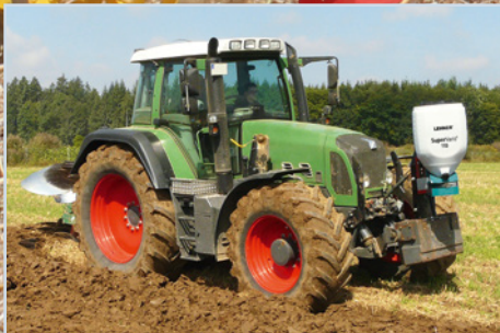
One-sided sowing of cover crops while ploughing
