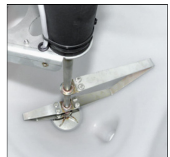
Saline agitator for slow-flowing materials – this agitator is not suitable for grit or sand.
