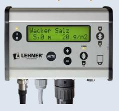
The menu of the AUTO-DOSIS control unit contains spreading charts from the manufacturer. If necessary, the manufacturer can install further spreading charts (if available).
