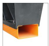
**Forklift shoes** (2x) for transporting and depositing the spreader.
