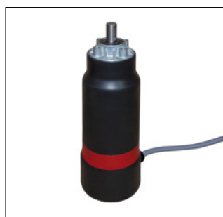
Spreading disc motor for larger working widths achieves a speed of 1,200 rpm and spreading widths of up to 12 m.
