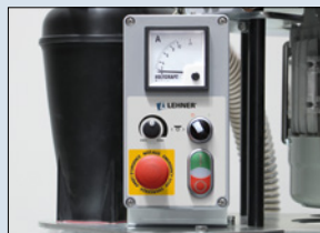
Control unit of the SpeltEx® with On/Off, Emergency Stop and ammeter.
