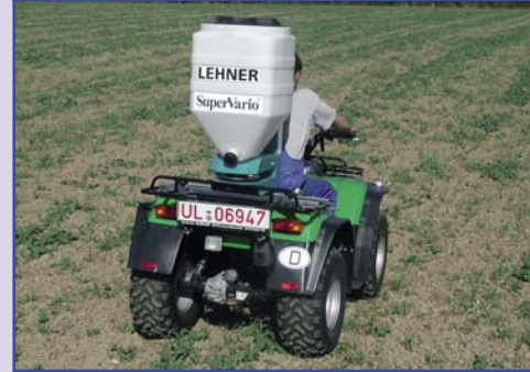
Spreading slug pellets with the ATV
